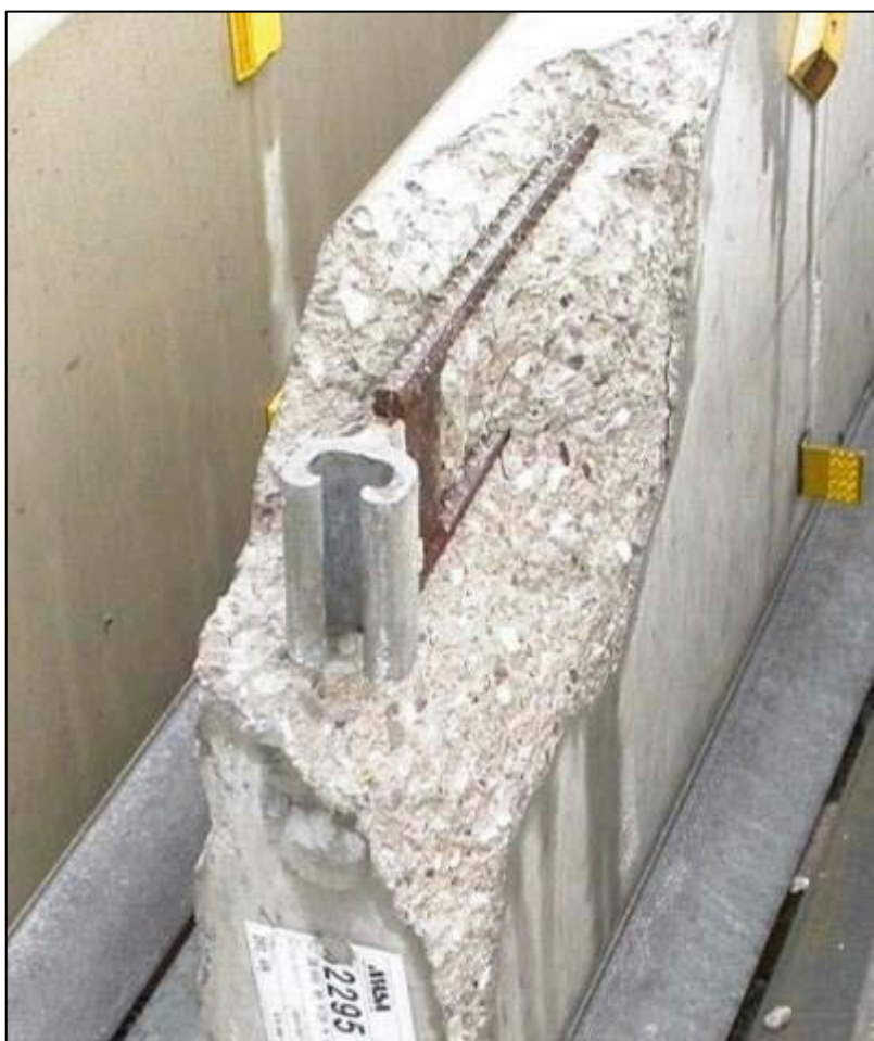
Figure 26: Exposure of Tension Bars
