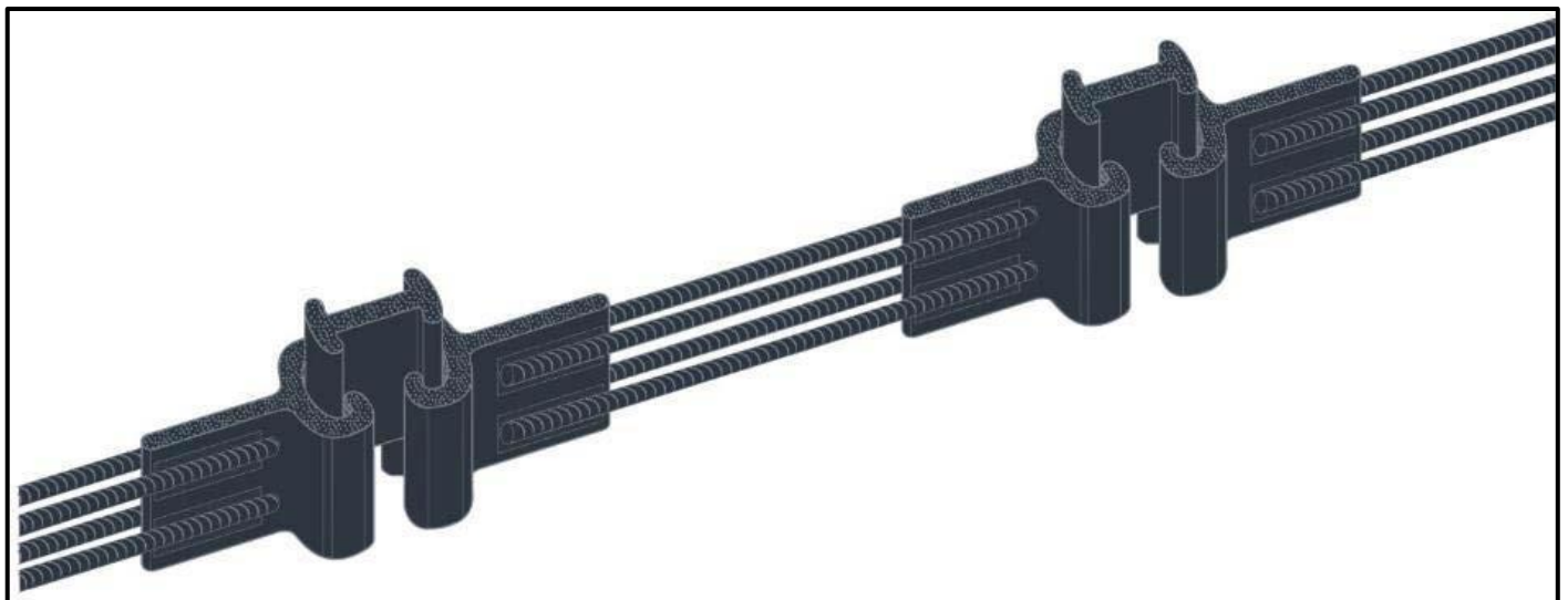
Figure 25: K-Coupling and Internal Tension Bar Arrangement
