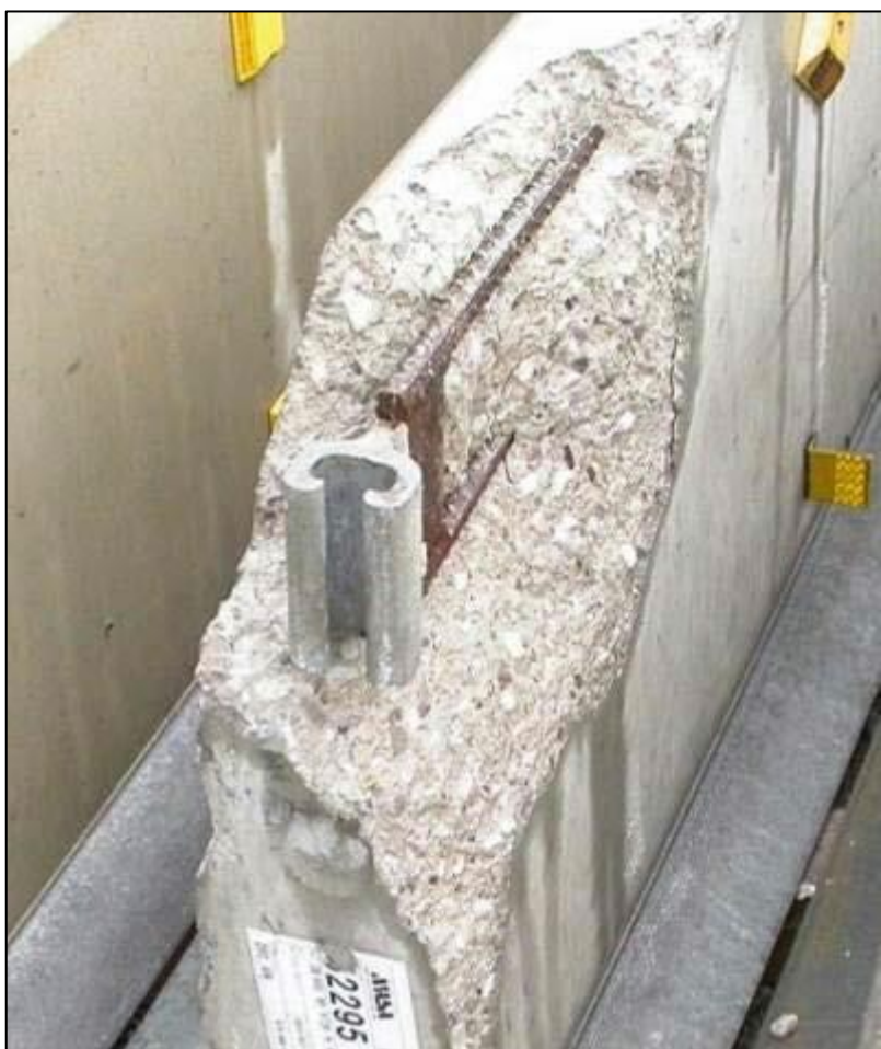
Figure 28: Exposure of Tension Bars
